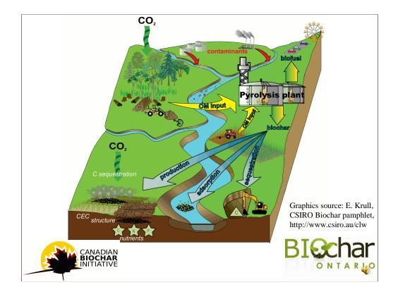
This is a depiction of **an** *Integrated* **Biochar system** Various carbon pathways can be integrated into a sustainable system with net **atmospheric capturing, safe use and storage**. Organic matter supplies for Biochar can include such things as:
